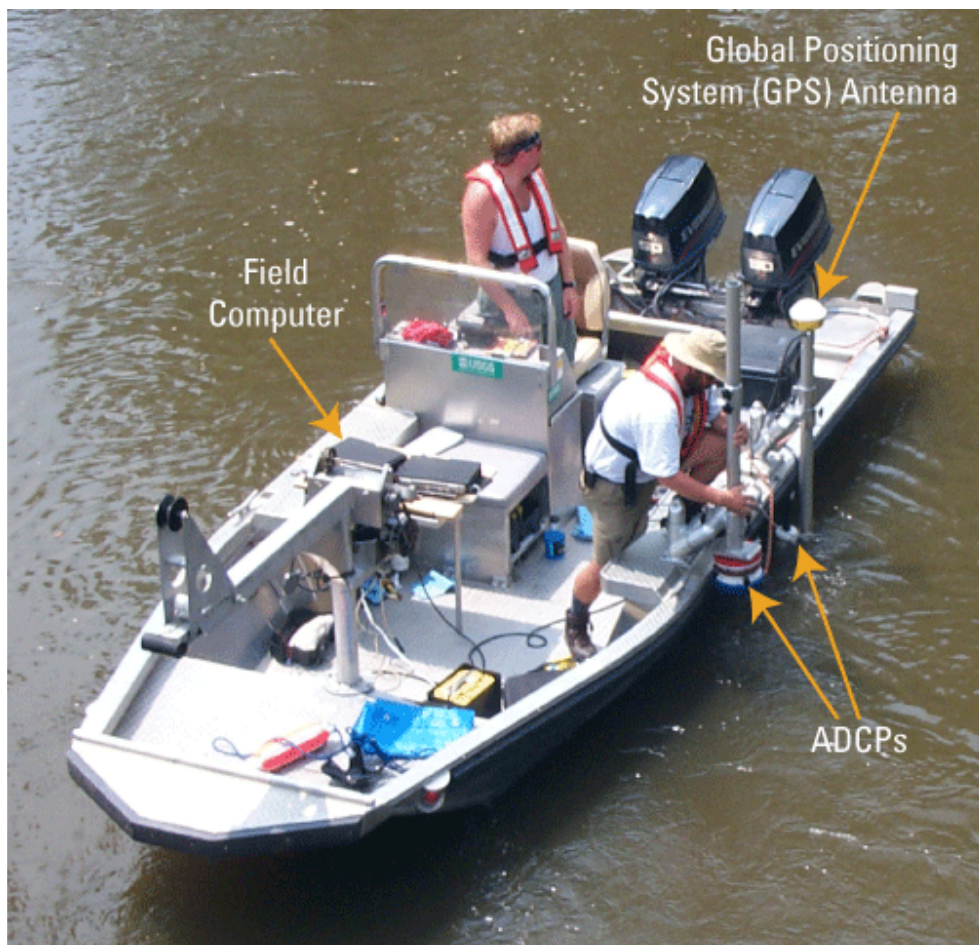
Figure 3. Side-mounted acoustic Doppler current profiler (ADCP) mounting brackets on U.S. Geological Survey work boat. (Photograph by Michael S. Rehm. U.S. Geological Survey.)
