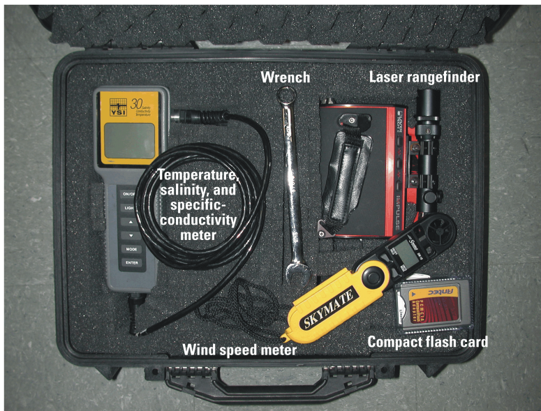
Figure 2. Example toolkit of ancillary equipment for use with acoustic Doppler current profilers (ADCPs) when making streamflow measurements. (Photograph by John M. Shelton, U.S. Geological Survey.)
